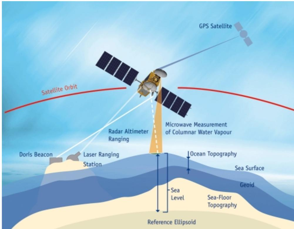
Satellite radar altimetry measures the time it takes for a radar pulse to travel from the satellite antenna to the surface and back to the satellite receiver. Apart from the surface height, this measurement yields a wealth of other information that can be used for a wide range of applications.
