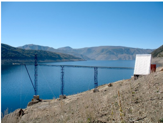
Figure 8: Starlab GNSS-R Sensor Oceanpal for monitoring lake level in ESA Business Applications project INTOGENER (/projects/intogener-feasibility-
