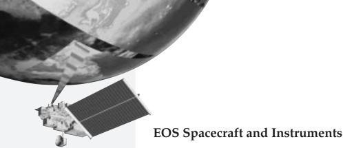
*ACRIMSAT* is a small satellite dedicated to the Active Cavity Radiometer Irradiance Monitor III (ACRIM III) instrument. ACRIM III provides long-term, precise
