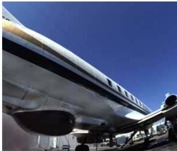
Black bulge under fuselage (radome) covers the radar antenna.
