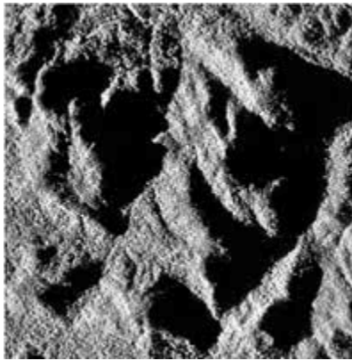
Example of radar shadow effects under large incidence angle (>45°) illumination.
