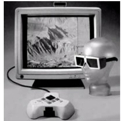
Digital Photogrammetric Workstation with a polarization screen and polarizing glasses
