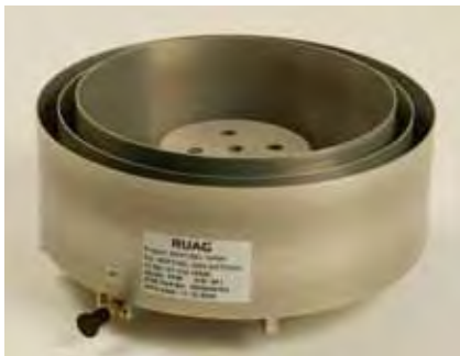
Figure 6.30. The two choke rings of the GPS antenna (diameter 200 mm). (TAS-F)
