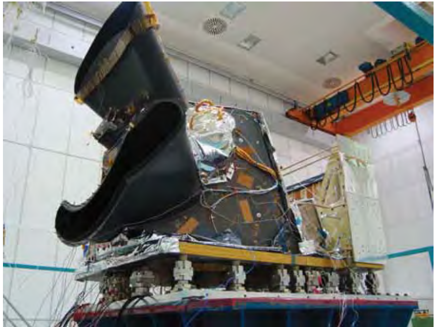
Figure 6.8. Structural and Thermal Model of the SLSTR, showing the large kidney-shaped Earth-view baffles of nadir (bottom) and oblique (top) views. (IABG)
