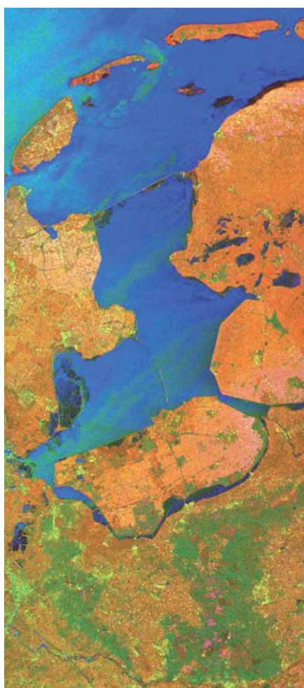
Revisiting a scene only a day later allows interferometry to distinguish between water bodies, forest, urban areas and agriculture. In this single ERS-1/ERS-2 image pair over The Netherlands, colours are assigned so that generally trees appear green, water appears blue and agricultural fields appear orange
