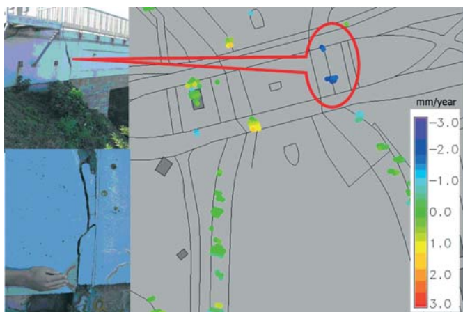
Detection by interferometric space radar of structural damage. The green spots show little movement, while the damage is highlighted in blue
