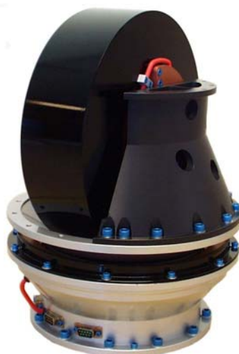
Figure 4-10: CMG mock-up of technology development
