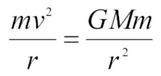
In this equation, m is the mass of the object in orbit, M is the mass of the Earth, r is the distance between the center of the earth and the object, is the velocity of the object, and G is a constant. If mass is measured in kilograms, velocity in meters per second and distance in meters, then G is equal to  $6.7259 \times 10^{-11}$ .
