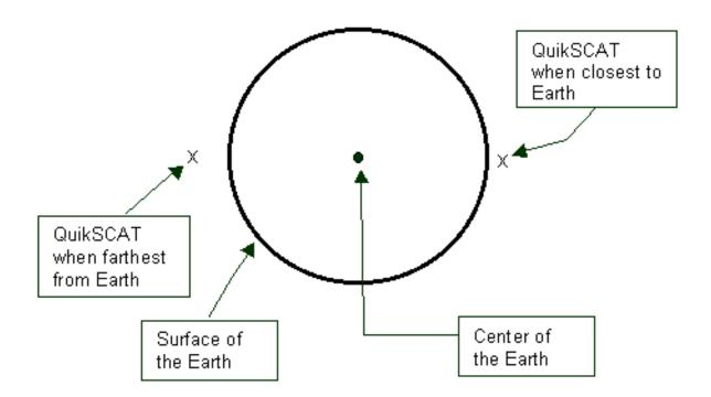
Since the Earth's radius is about 6000 kilometers, that means the QuikSCAT's orbit was 6200 kilometers from the center of the Earth at its closest, and 6800 kilometers from the center of the Earth at its farthest distance. This sketch shows these two positions (note that the radius of the Earth is 6000 kilometers).
