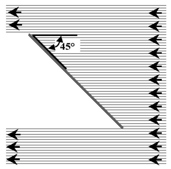
In the first diagram, the incoming radiation arrives at an angle of 90° to the face of the solar panel. In the second diagram, the angle is 45°.
