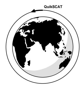
We have put the QuikSCAT satellite into a circular orbit. Is there a relatively easy way we can determine the speed at which a satellite moves in its orbit? The answer is yes, if we know its distance from the center of the Earth (or visa a versa).
