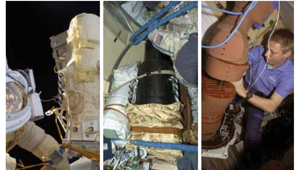
Figure 1: The MATROSHKA facility: (a) outside ISS exposure (simulation of a spacewalk) MTR-1 experiment phase; (b) inside ISS exposure MTR-2A experiment phase; (c) European astronaut Thomas Reiter removing the radiation detectors after the experiment phase MTR-2A for read out and data evaluation on ground. © NASA
