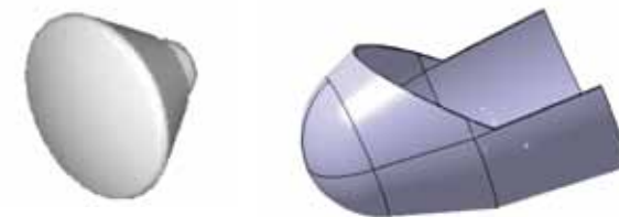
Figure 1: Two different shapes for the aerocapture system are currently under assessment from the system and design point of view: ARD-like (sphere-conical shape) and a biconic shape
