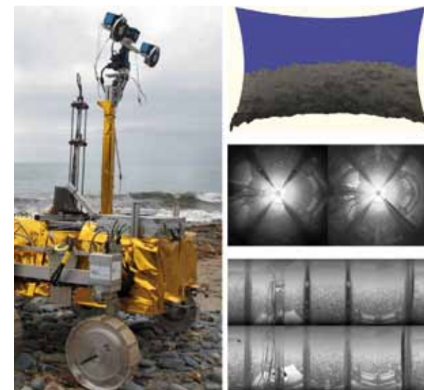
Figure 1: Left: CSEM Catadioptric sensor & 3D-Time-of-Flight (3D-TOF) camera mounted on ASU Bridget Rover during field test at Clarach Bay, Aberystwyth, July 2010 © Joanneum Research. Right: (top) 3D-TOF distance image (grey coded), (middle) catadioptric sensor images and (bottom) reconstructed panorama from catadioptric sensor © CSEM
