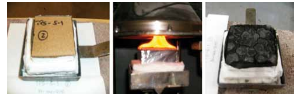
Figure 2: Sample of thermal protection before, during, and after testing
