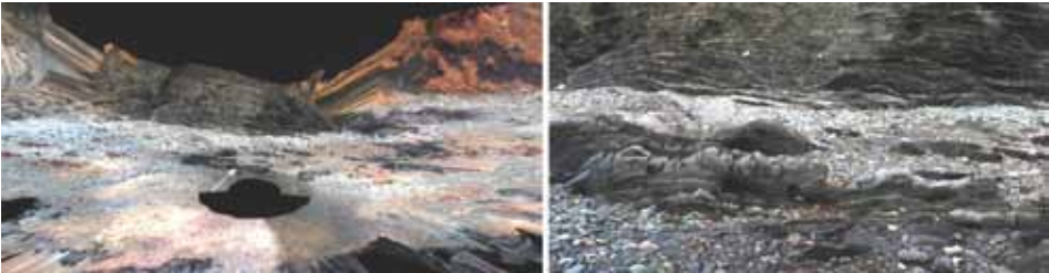
Figure 3: Rendering of 3D reconstruction using ExoMars PanCam – simulating stereo, 20 pairs. Left: Whole area in viewer. Right: Close-up at the marked position in the overview. A high resolution video showing real-time rendering of this area is available at YouTube. Credits: VRVis, Vienna. © Joanneum Research
