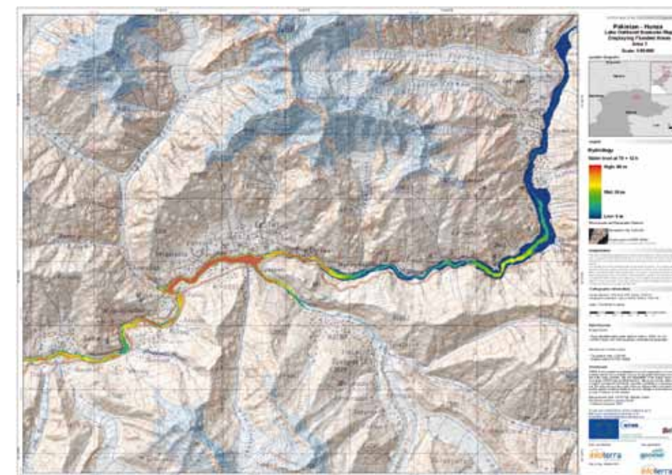
Figure 4: Map showing results of modelling dam breach and flood wave progression
