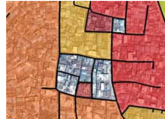
Figure 7: Port-Au-Prince Damage Assessment derived from point layer of destroyed buildings - © Digitalglobe 2010 provided by e-Geos under EC/ESA GSC/DA
