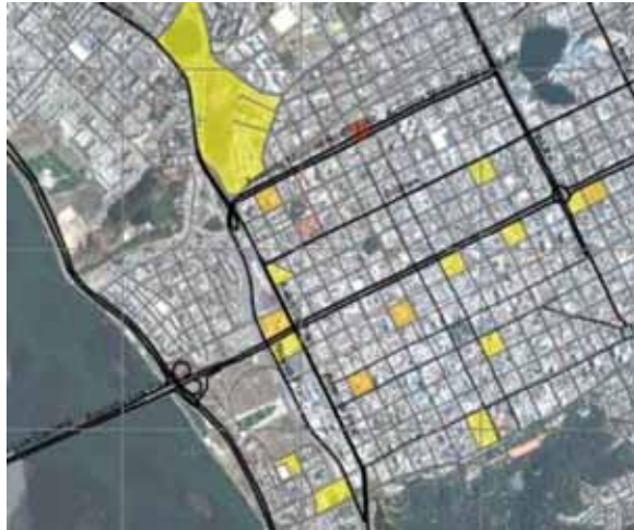
Figure 4: Urban Block damage assessment orientated to represent the damage of the earthquake produced by RGR. © Digitalglobe 2010 provided by e-Geos under EC/ESA GSC/DA
