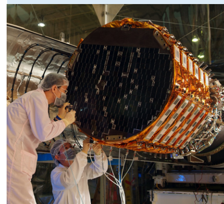
Six FORMOSAT-3/COSMIC satellites mated to the Minotaur launch vehicle
