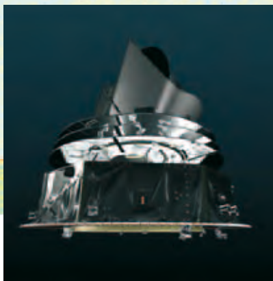
The bottom of the satellite is warm and contains all the electronics and other subsystems.
