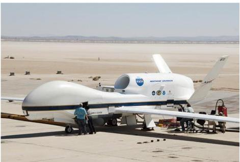
Land-based and airborne instruments complement NASA's satellites. AERONET is a global network of sun photometers that measures aerosols from the ground, such as this station in the Canadian Arctic (top). The Global Hawk Uninhabited Aerial Vehicle (bottom) can carry several instruments to measure aerosols from the air. Photograph by Ovidiu Pancrati, ©2007 CANDAC. Lower photograph by Tony Landis/NASA.)
