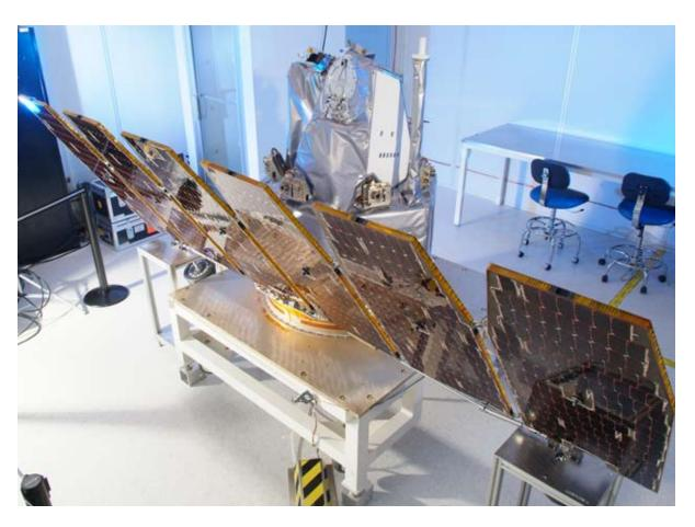
This is the AIM spacecraft with the solar array fully deployed. There are six separate solar array panels, which are integrated into a single deployed wing. In this orientation the nadir deck is pointed up towards the ceiling, and the SOFIE and CIPS instruments are visible in the photo. The photograph was taken in the clean room at the Orbital Sciences Dulles, Va. facility.
